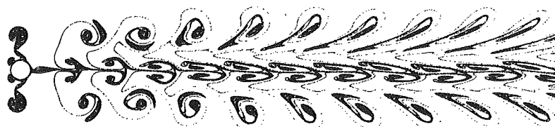
Fig. 9 Oscillatory plus mean flow about a circular cylinder and the evolution of three rows of heterostrophic vortices ( K = 4 , Re = 800 , V_r/U_m = 0.65 )
